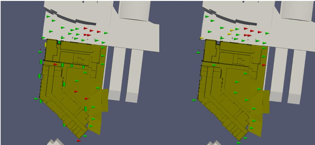
**Figure 5.8: Comparison of Lawson Comfort Criteria for Block 17 without (left) and with mitigation (right)**
