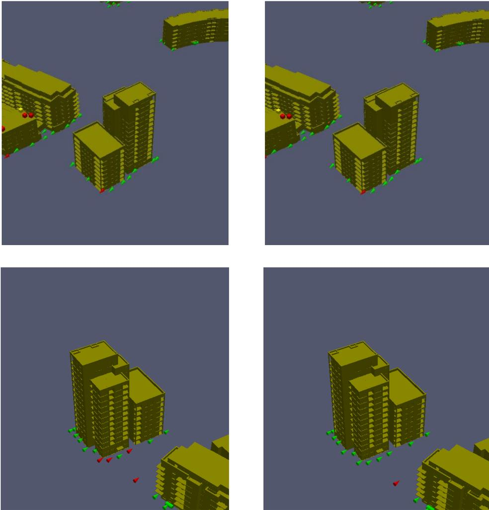
**Figure 5.9: Comparison of Lawson Comfort Criteria for Block 26 without (left) and with mitigation (right)**
